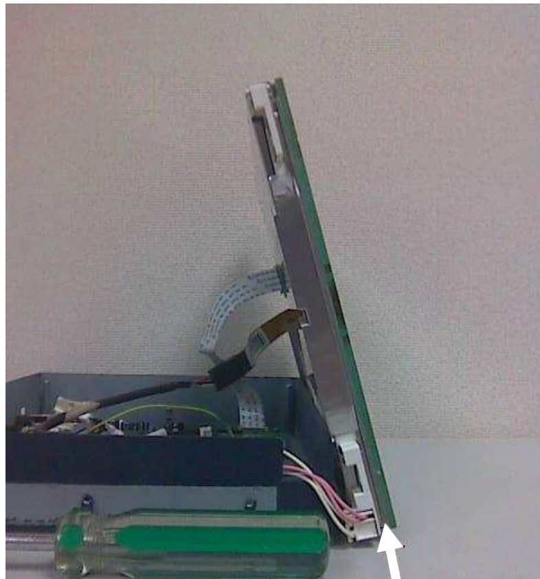
Sponge tape between touch panel and LCD monitor
